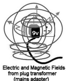
Sometimes transformers are built into radios and music players and are actively emitting magnetic fields all the time the player is plugged into the mains, even when it is not actually in use.
