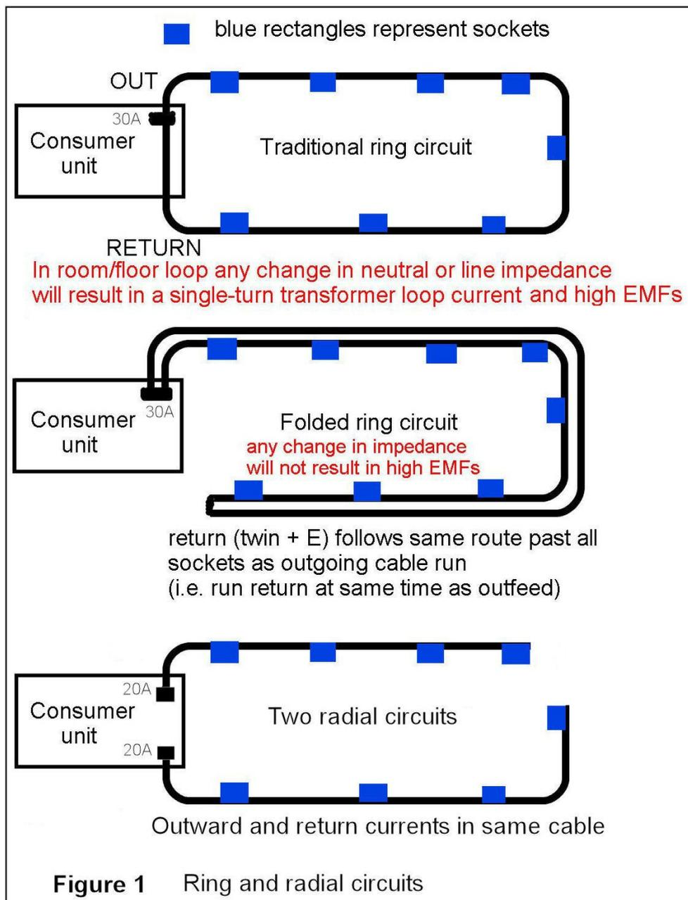
In the worst case, which is surprisingly common, a Line or Neutral actually gets disconnected (often as a result of incompetent DIY) and this effectively results in a single-turn transformer loop. When a significant load is applied, the magnetic field in rooms throughout the inside of the ring can rise to many microtesla.
