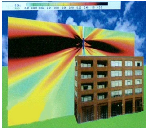
A base station on the roof of a building, showing signal strength levels
