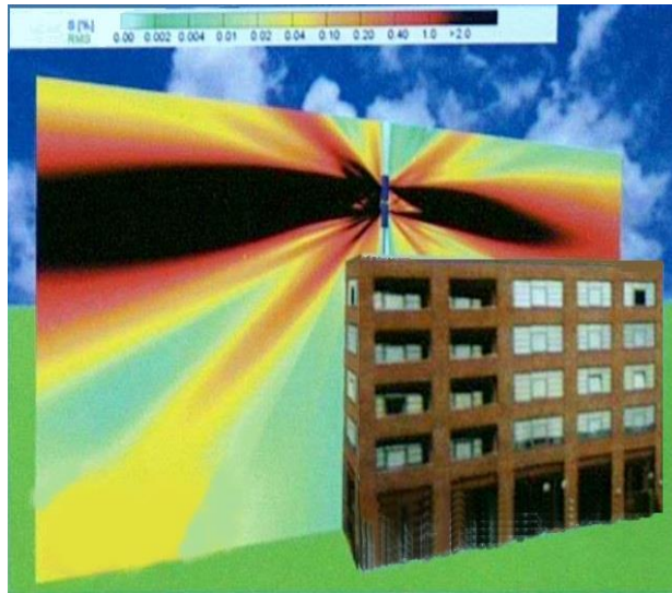
A base station on the roof of a building, showing signal strength levels
