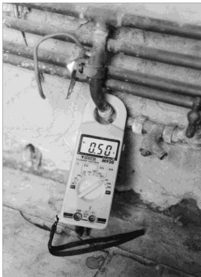
0.5 Amps stray current flowing on incoming main cold water pipe
