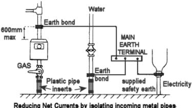
Reducing Net Currents by isolating incoming metal pipes
