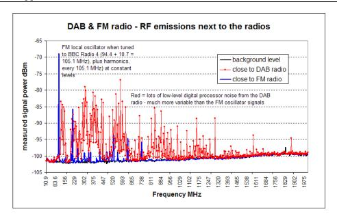
As can be clearly seen on the graph, the DAB radio emits far more noise over a wide range, although the FM radio peaks at a higher level.
